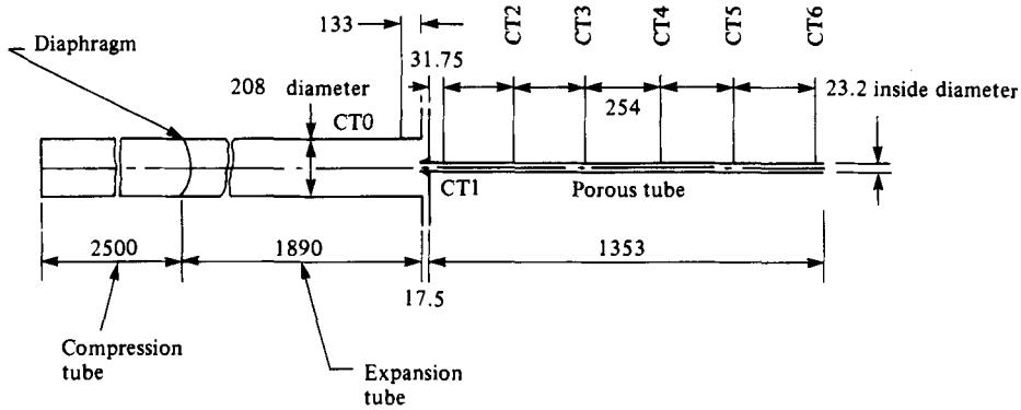
FIGURE 1. Schematic drawing of shock tube (dimensions in mm).
