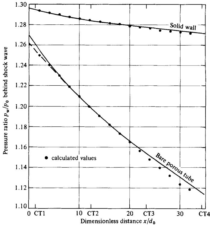
FIGURE 5. Spatial decrease in pressure ratio behind shock wave in a bare porous tube and in a tube with solid walls showing comparison between experimental curves, from figure 2(a), and calculated values from quasi-steady analysis.
